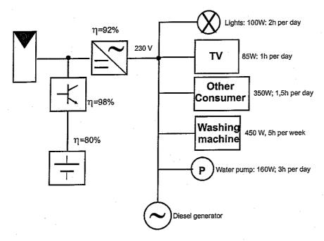
He bought a PV generator of 150  $W_{pk}$  and a battery system, which is adjusted to the size of the PV generator. All generated PV power will be consumed within the system.
